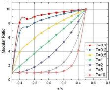
Fig. 5. The variation of Modular ratio in a P-FGM shell
