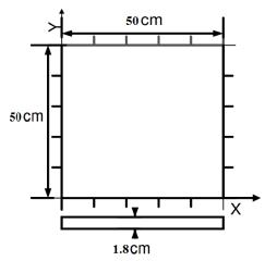
Fig. 4. Simply supported rectangular shell
