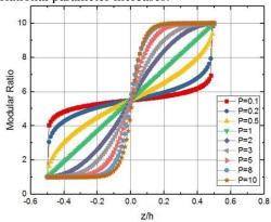
Fig. 6. The variation of Modular ratio in a S-FGM shell
